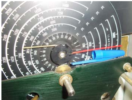
Right pointer wheel repaired and re-installed.
