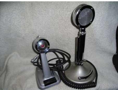
Picture 3: (L) A Turner crystal desk mike from 1969; (R) Astatic D-104 crystal mike.
