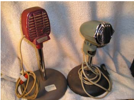
Picture 2: (L) Shure 710A crystal mike from 1949; Ar-gonne M-31 Japan crystal mike from 1965
