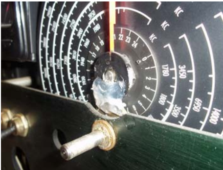
Right pointer wheel repaired and re-installed.
