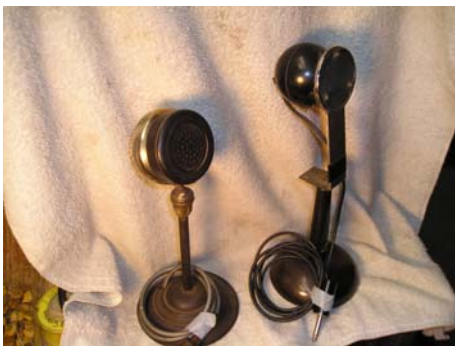
Picture 1: (L) Western Electric carbon mike from 1920's; (R) Western Electric 630 (moving coil dynamic) from 1935 also called the "Eight Ball"
