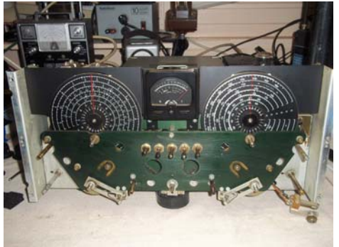
Right pointer wheel repaired and re-installed.
